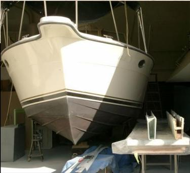
New fiberglass molded stringers being fitted to replace the built-in rotted plywood stringers on this 31' Twin Inboard
