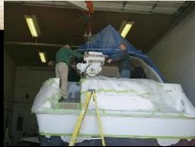
Removing the diesel engine from a 45' twin diesel inboard to facilitate structural repairs
